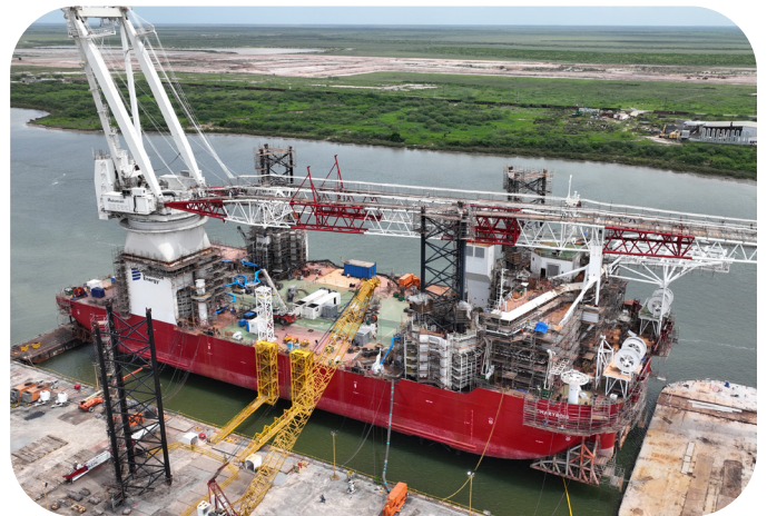
CHARYBDIS VESSEL: The Charybdis is the first U.S.-built wind turbine installation vessel, a valuable asset for future offshore wind construction beginning with Dominion Energy's Coastal Virginia Offshore Wind project in the summer of 2024.
